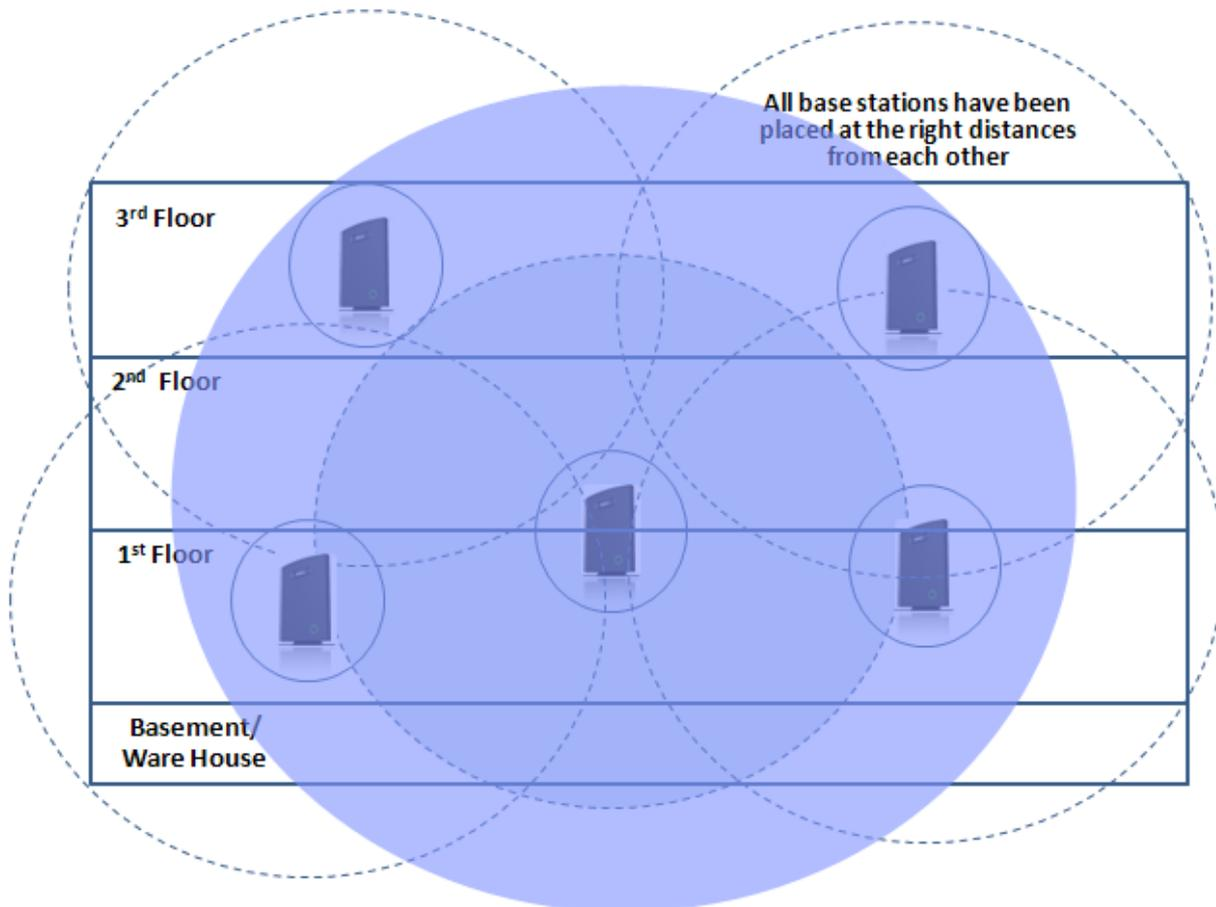
Typically, installations such as office buildings, hotels and hospitals should be equipped with both base stations and repeaters on several floors to create uniform and complete radio coverage.
