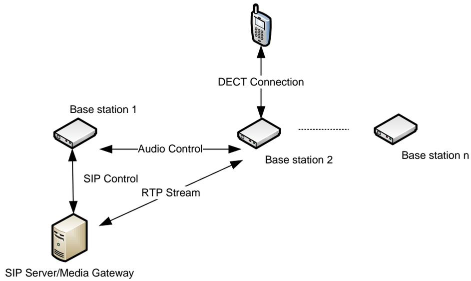
An illustration of Handset moving to another base station, but call control is still handled by the initial base station.
