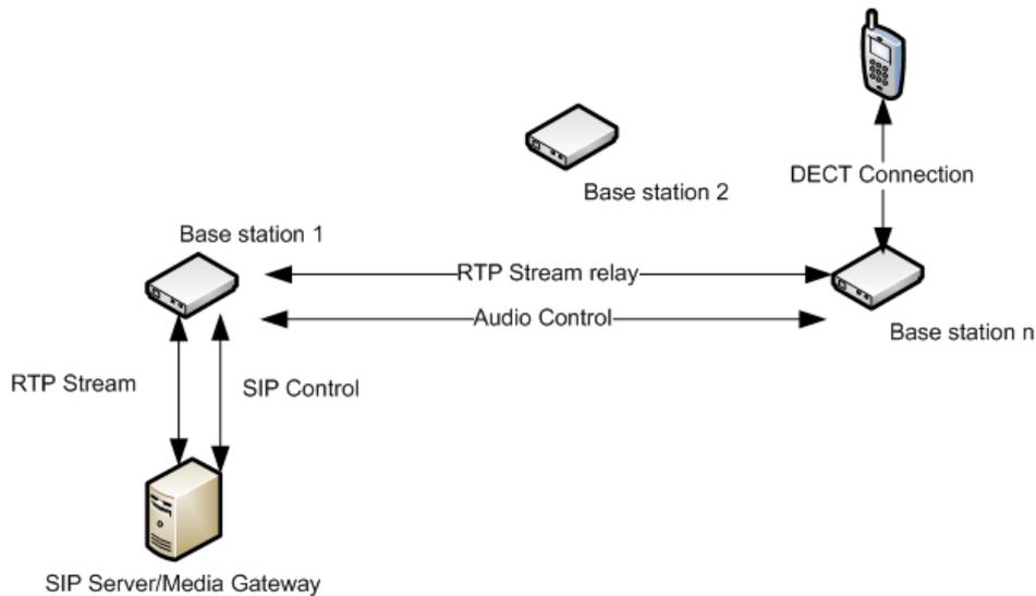
**After handover to BS *n* the handset is located at BS *n*, and the RTP stream is relayed via BS 1.**
