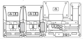
Note: The T52S/T54S/T56A/T58A/T58V IP phone can support 3 expansion modules at most. But if you use more than one expansion module, you need to connect an additional Yealink power adapter (5V/2A) to any one of the expansion modules. The power adapter should be purchased separately.
