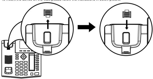
Figure 2 - Change handset hook to wall-mount mode
