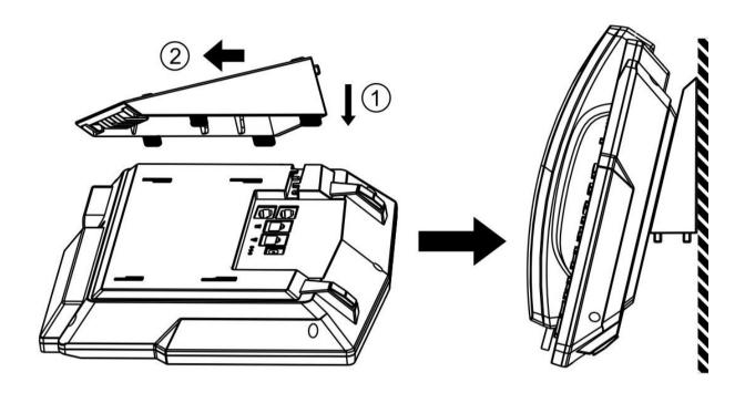
Figure 3 - Wall-mount Installation
