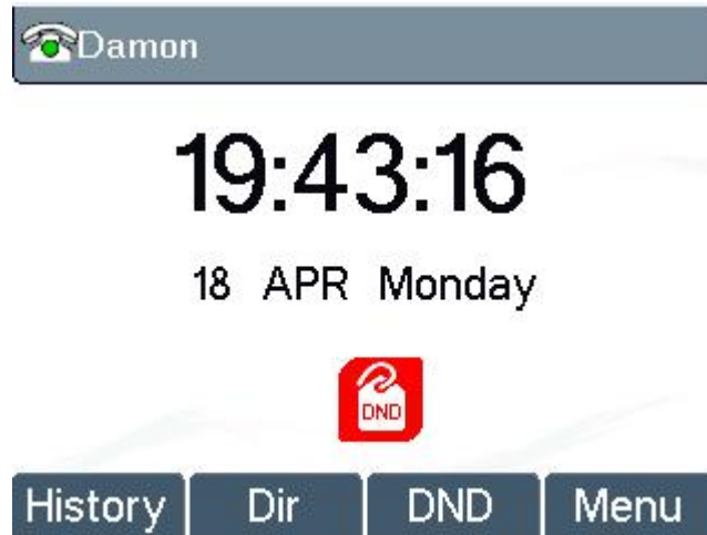
Figure 57 - DND Enabled on All Lines
